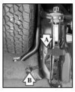
2. Turn the wingnut (A), which holds the jack, counterclockwise to release the jack.
